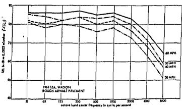
FIGURE 12 Noise Spectra for a Passenger Car at Four Speeds
