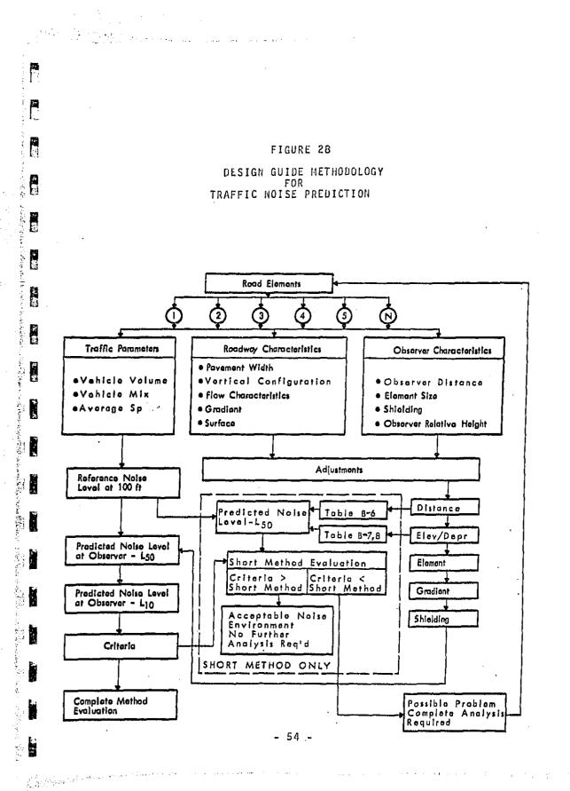
The use of the Design Guide method requires identification of roadway elements with constant geometric characteristics. Each element that is identified is then described by a series of parameters. The parameters required for utilization of the method can be grouped as follows:
