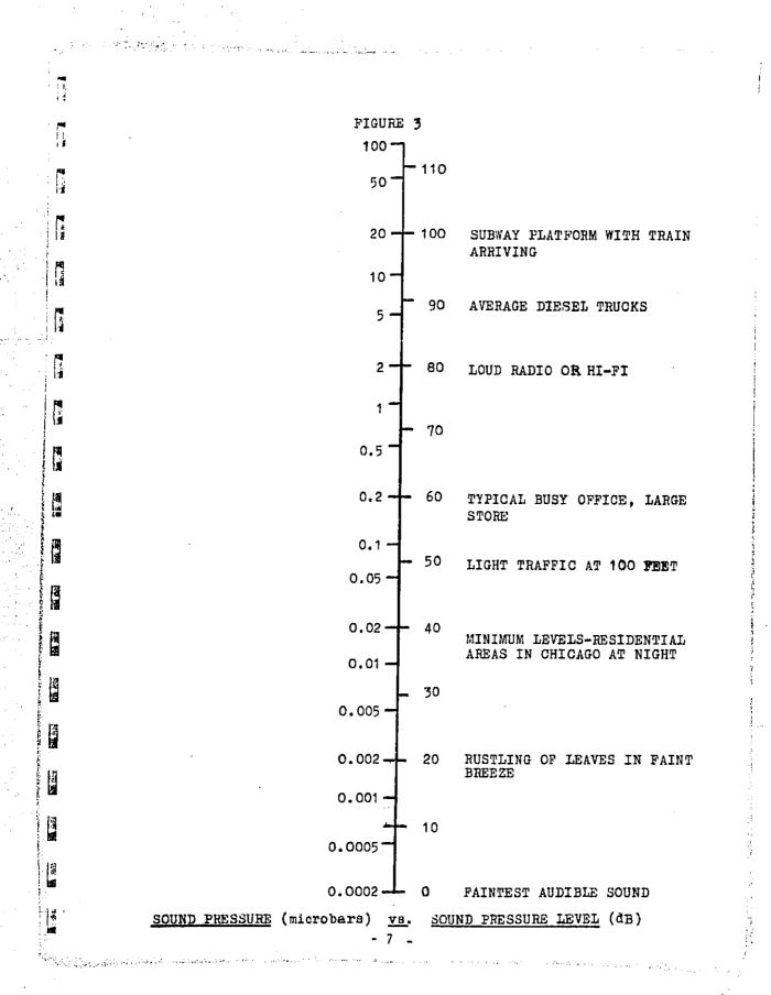
Figure 3 Various easily identified sounds are included in Figure 3, next to their corresponding levels.
